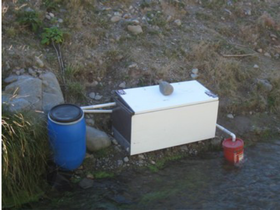
Fig 2. The set-up: blue filter barrel, alevinator and catch bucket.
