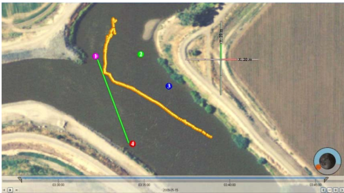
Figure 6. A juvenile Chinook salmon (tag # 5674) approaches the BAFF (green line). The tag exhibits a smolt-like trace: downstream quickly and no predator behavior. The colored circles indicate the location and number of the four hydrophones. Reproduced from Bowen et al. (2009).
