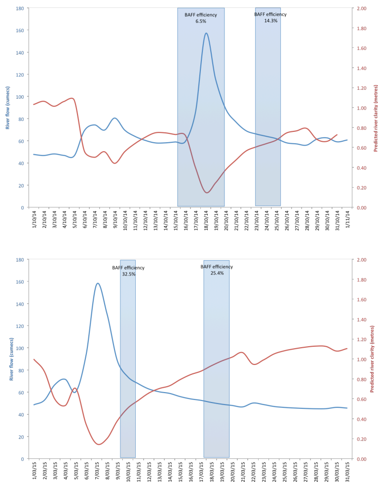
Figure 3. Recent estimates of BAFF efficiency (at deflecting salmon smolt) compares against Rangitata River flow and estimated water clarity during the trials.
